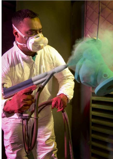
Applied Plastics electrostatically spray coats items ranging from needles to tool handles, machine housings to chemical valves, and large castings weighing up to 4,000 lbs. After spraying, they are cured in an oven at temperatures from 200°F to 800°F, for varying durations, depending upon the item and coating. We can effectively coat individual pieces, short runs, or high-quantity production runs.
